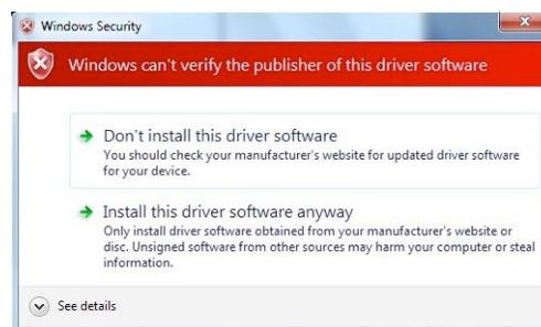
(9) The message displayed below is a reminder to Re-launch Linkmotion one time after installation is finished for the driver to be recognized properly and Click on the OK button here. **Make sure to click on the OK button after you click on the “Install this driver software anyway”.**
