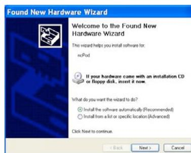
7. On Win 8 and 7 first dialog box shown above will be displayed and it can automatically search and then install the driver from your computer. The user can save time by clicking on the message **Skip obtaining driver software from Windows Update** and click Yes on the next message (picture not shown). On Win XP Found new hardware wizard dialog box shows up and make sure to check the button for **Install software automatically (Recommended)**. **Click on the Next button.**
