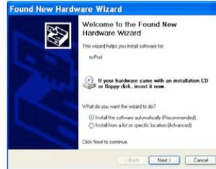
7. Found new hardware wizard dialog box shows up and make sure to select the button for **Browse my Computer** for Win 10, 8.1, 8 and 7 or **Install the software automatically (Recommended)** for Win XP. Click on the Next button. Do not allow for windows to look for the driver on the internet.
